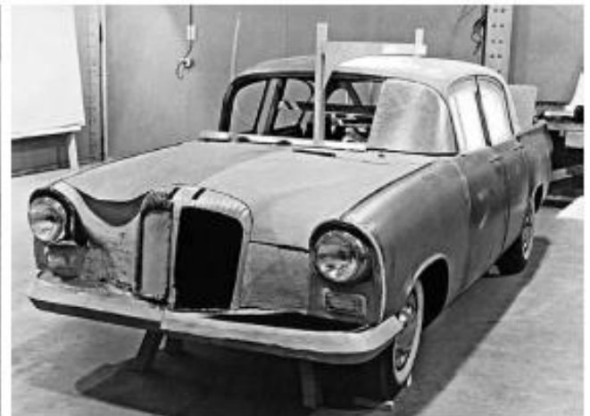
A flying mock-up of the proposed Daimler DN250 V8 Saloon based on the Vauxhall Cresta PA Series bodyshell
