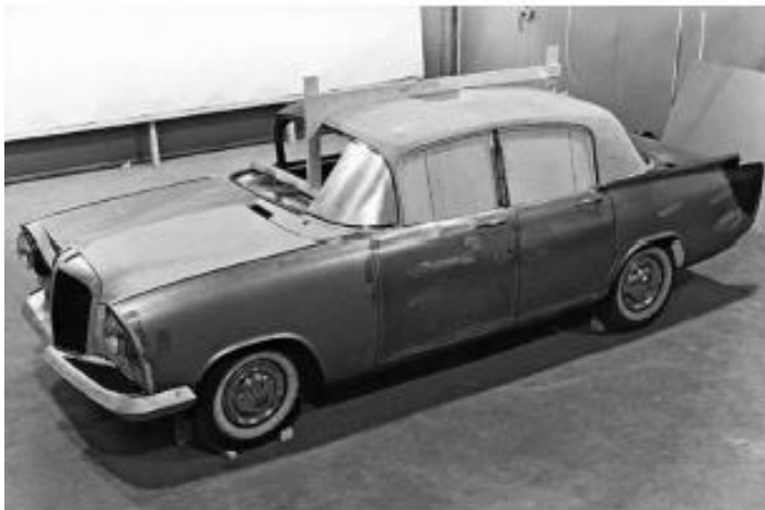
A wireframe mock-up of the proposed Daimler DN250 V8 Saloon based on the Vauxhall Cresta PA Series bodyshell
